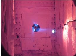
Typical burner construction includes various metal components and a refractory throat or tile. The increased flame temperature of  $H_2$  requires upgrading the steel used for nozzle construction, throat construction, and flame stabilizers to a higher
